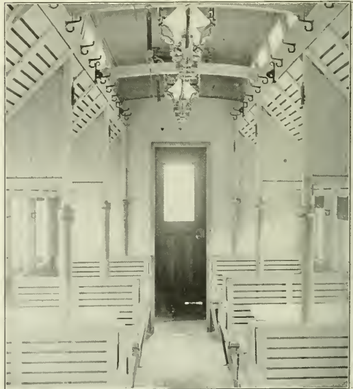
Sleeping Car for Use in Wrecking Trains.
